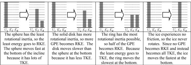
If an object rolls down an incline and slips, then pat of the GPE turns into TKE+RKE, but some of the energy is lost to frictional effects.
