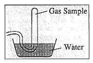
A student collected a sample of hydrogen gas by the displacement of water as shown by the diagram above. The relevant data are given in the following table.
