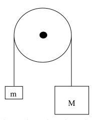
16. Assuming the pulley above is frictionless and massless, determine the acceleration of the blocks once they are released from rest.
