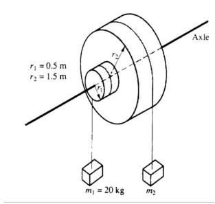
The mass m<sub>2</sub> is removed and the system is released from rest.
