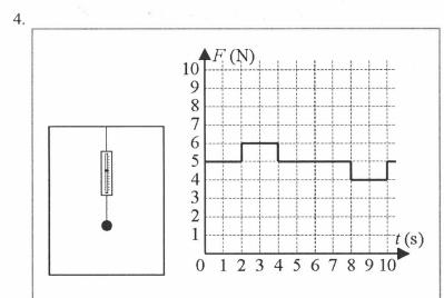
A known mass hangs from a force sensor inside of an elevator. As the elevator moves from the bottom floor to the roof-level of a building, the upward force acting on the mass is recorded as a function of time in the graph shown. Which of the following questions could NOT be answered by the data in the graph and the known mass?
