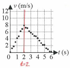
A 6 kg block is set on a rough table and connected to a hanging mass by a string that passes over an ideal pulley. The system is released from rest at time t = 0, and the block speeds up as the mass falls. Once the mass strikes the floor, the block comes to rest again. A student uses measurement apparatus to collect data of the block's velocity as a function of time. The data are shown in the graph above right.
