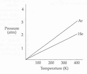
The graph above shows the changes in pressure with changing temperature of gas samples of helium and argon confined in a closed 2-liter vessel.
